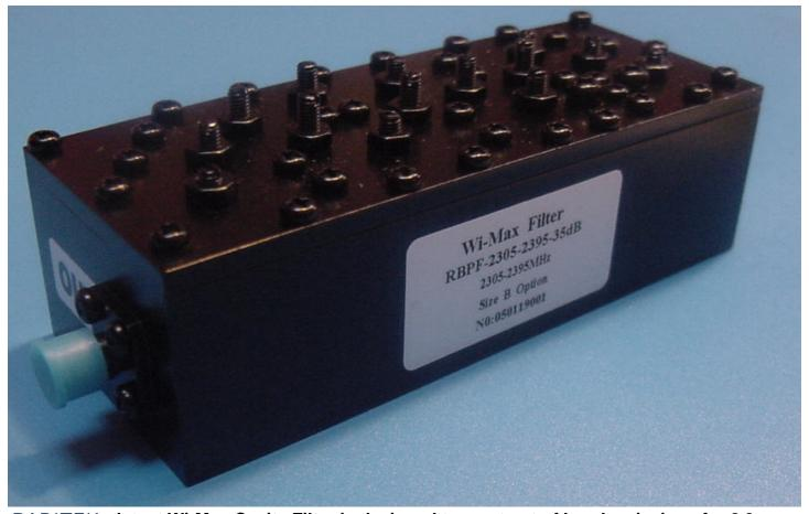
RADITEK's latest Wi-Max Cavity Filter is designed to meet out of band emissions for 2.3-2.4GHz Wibro / Wi-Max transmissions; this compact filter is placed between the TX/RX module and the antenna. 1dB Pass band 2305-2395MHz and > 60dB rejection 2030-2250MHz and 2450-2670MHz, Average power handling is 4Watts and 50Watt peak. These units are proven in the field and are fully ROHS compliant.
